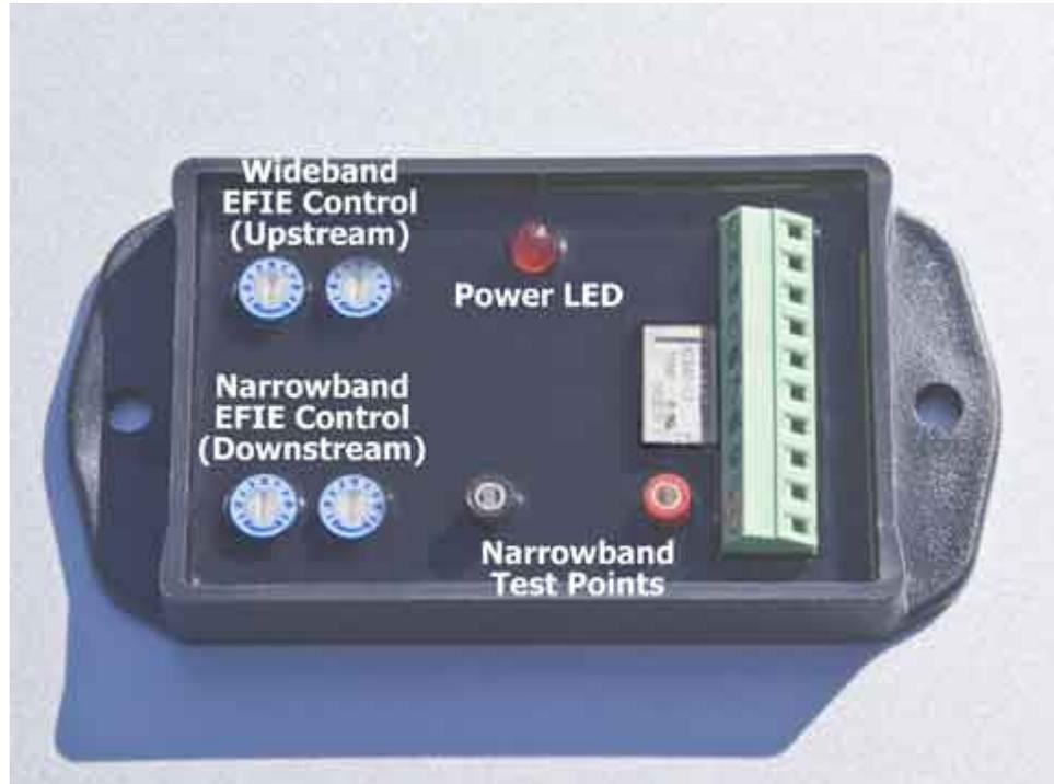
The Wideband Dual EFIE has the same controls as the Wideband Quad EFIE. However, the Dual model has only one of each type of EFIE whereas the Quad has 2 of each type..
