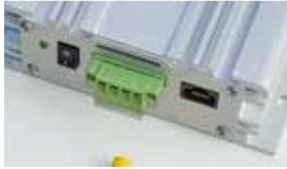
There is a small green pluggable terminal block used for low current connections to the PWM. It's easiest to unplug the terminal block and then install the wires. When you are done, plug the terminal block back in. There are screws you can use to secure the block into the PWM.
