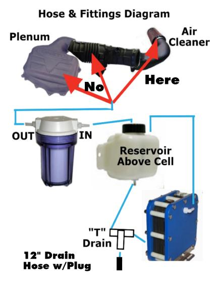
Complete the hose connections to all the devices as shown in the diagram.
